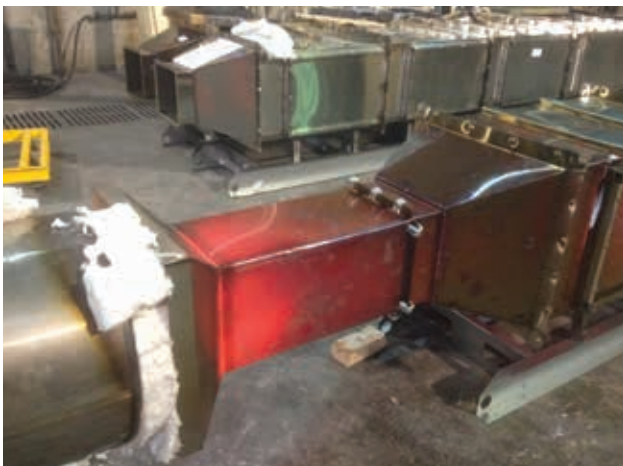
Abnormal Temperature Test PCU must completely contain all smoke and flame to pass UL 1978 test standard. Greenheck unit passed all UL 1978 est criteria.
