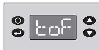
Minimum Cooling Temperature Display
